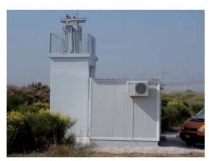
aircraft emissions during takeoff. Data from DOAS are available from October 2005 onwards. Seven pollutants are measured: nitric oxide, nitrogen dioxide, ozone, sulphur dioxide, benzene, toluene and xylene, as well as the basic meteorological parameters (wind speed and direction, temperature and relative humidity).
